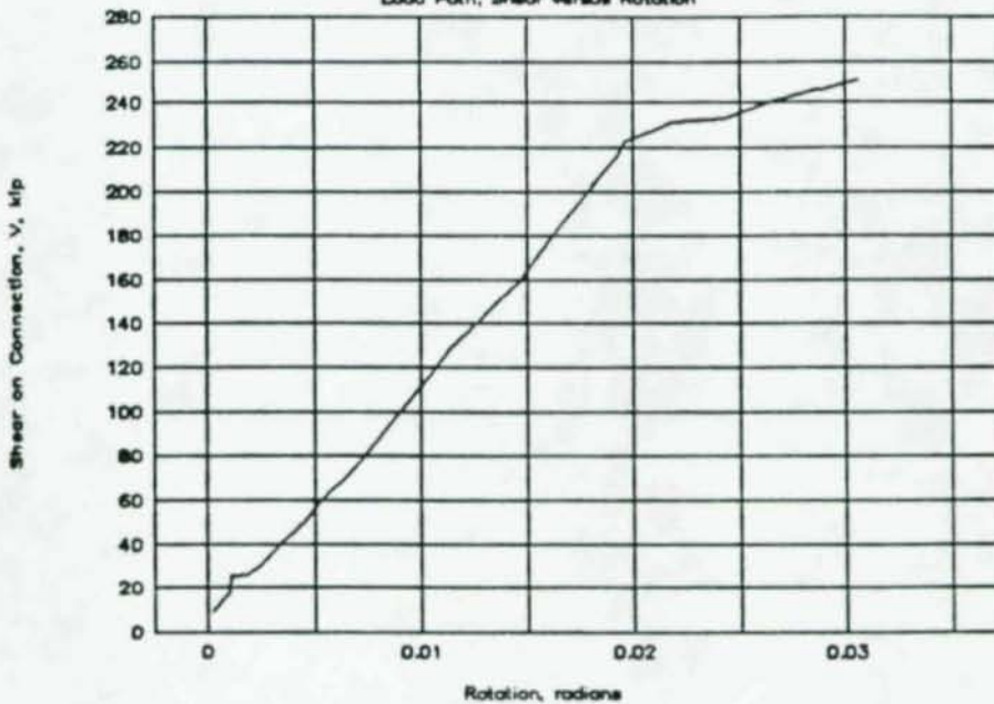
Figure A-4: Load path for 9-bolt specimen
