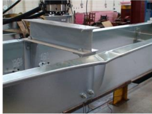
Local buckling (Experiments: ZB63-C e ZC83-C)
