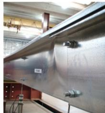
Local buckling of the purlin at the connection end
