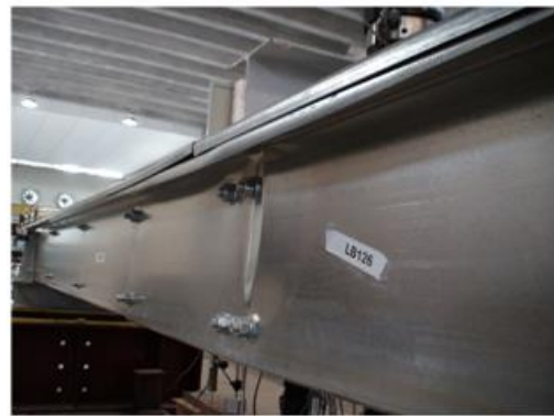
Local buckling at the middle of the sleeve
