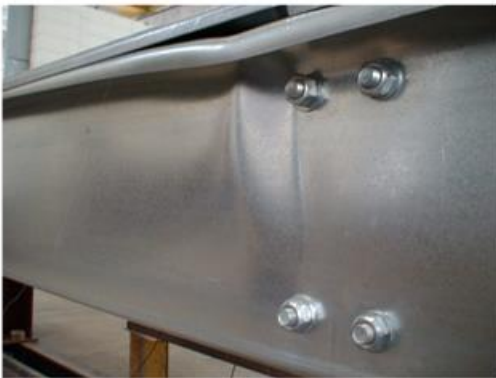
Local buckling at the middle of the sleeve
