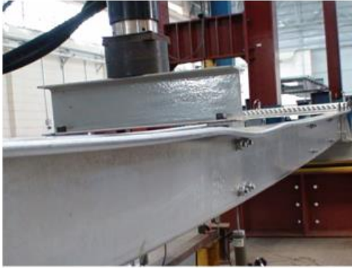
Distortional buckling (Experiment: ZA62-C)
